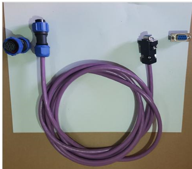
Connection between MD-0x controller and rotator with optional ABS sensors
